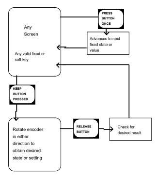
Fig. 2.1 Setting and Parameter Entry Flowchart
