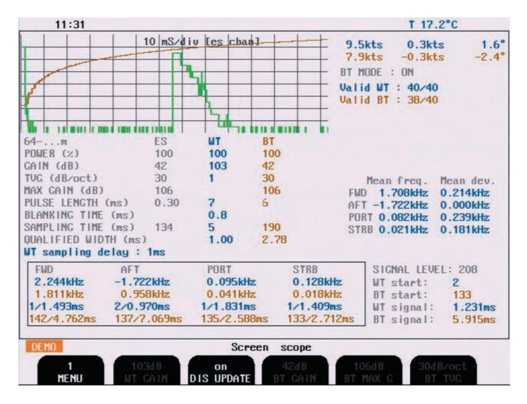
The scope screen will differ depending if a three beam or a five beam sensor is istalled. Screens here are shown with five beams.
