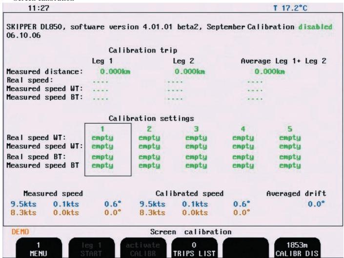
The various soft key menus are selected by pressing repeatedly the MENU button on the left side of the soft key menu. The number on the button indicates which of the menus is active.
