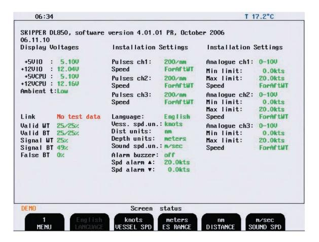
If it is at all possible to cycle through the screens and observe this information, several assumptions may be made regarding operation of the DL850 System. Although some of the subsystems necessary for this basic system operation may still suffer from minor or intermittent operation disorders, the fact that it is possible to select and observe this screen, indicate correct operation of the following DL850 Subsystems:
