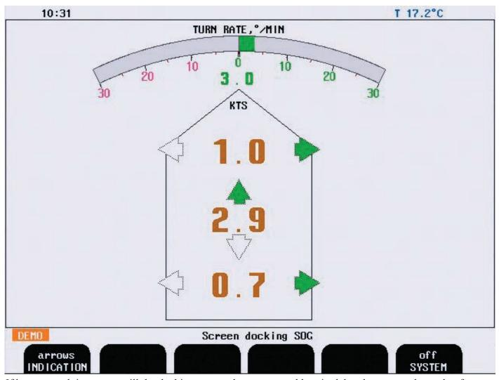
If bottom track is present will the docking screen show measured longitudal and transversal speed at fore and calculated speed at stern point.
