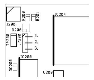
Fig. 4.5 History Memory Battery Jumper, I/O Board.
